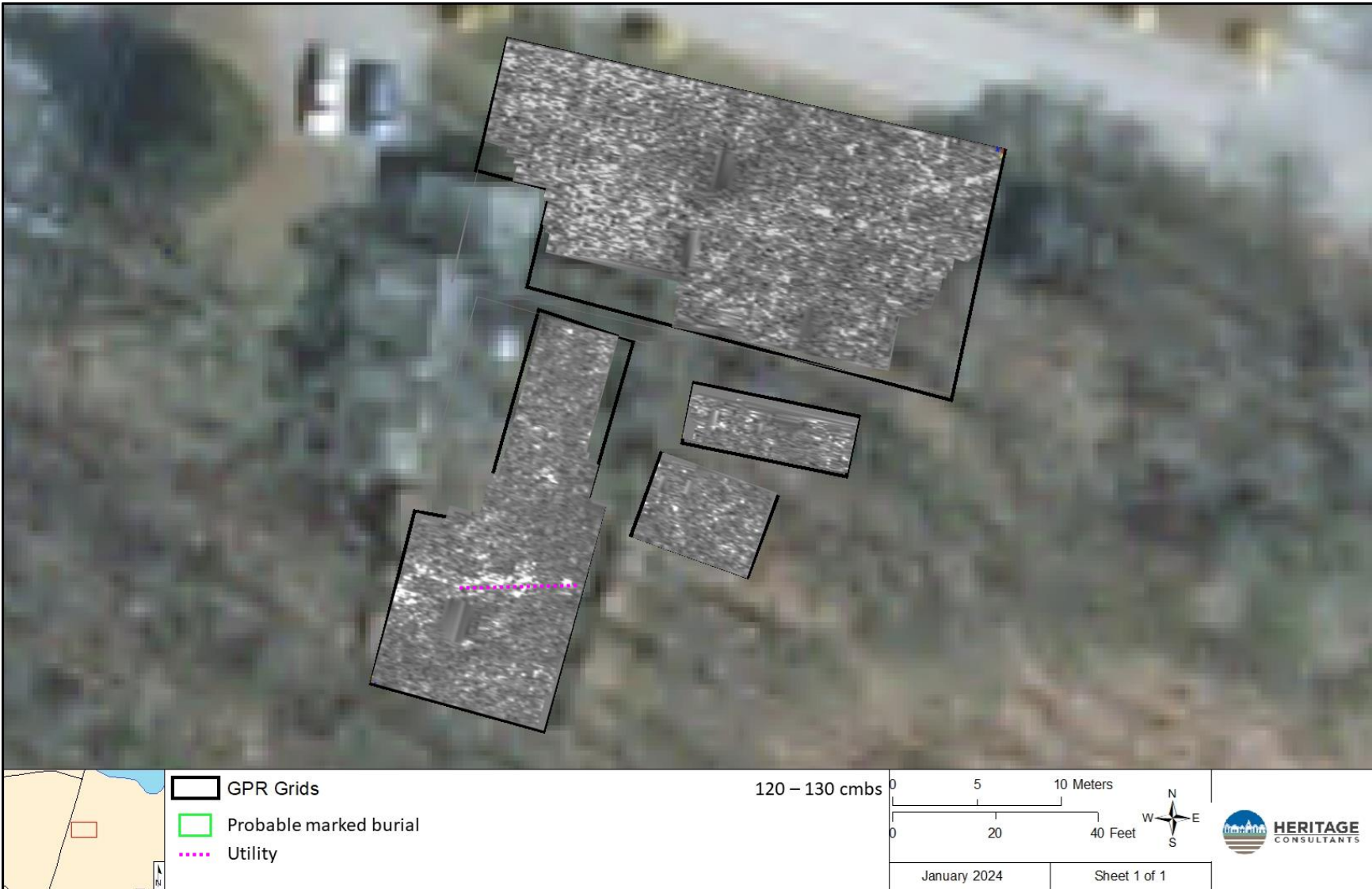
Figure 44: Annotated GPR amplitude map of Survey Grids 1-4, with approximate depth indicated.
