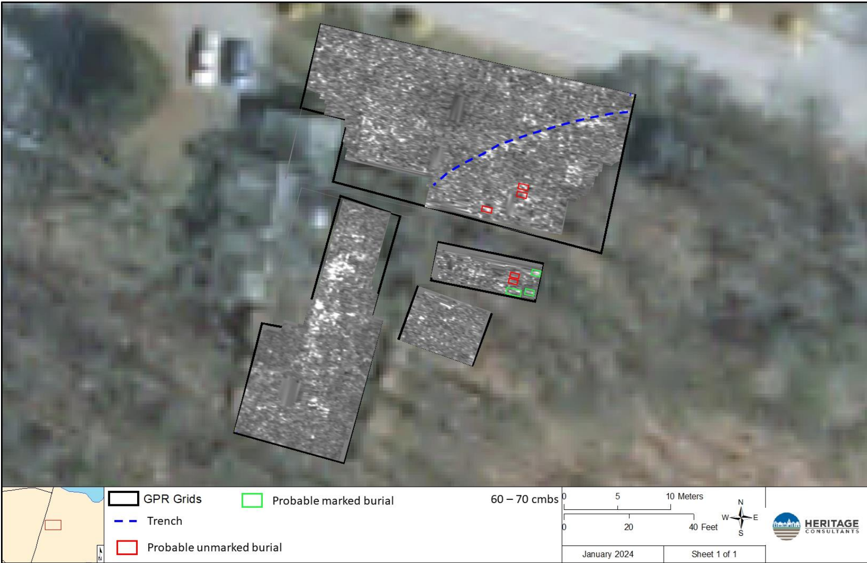
Figure 38: Annotated GPR amplitude map of Survey Grids 1-4, with approximate depth indicated.
