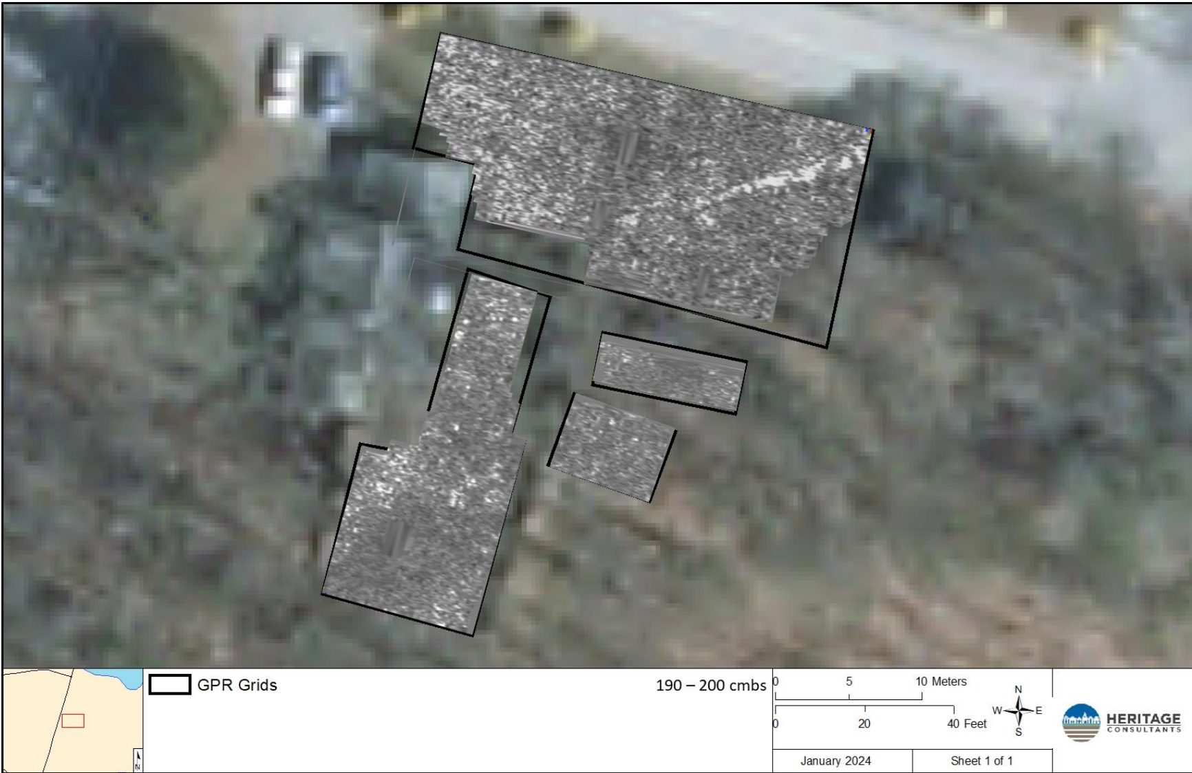
Figure 31: GPR amplitude map of Survey Grids 1-4, with approximate depth indicated.
