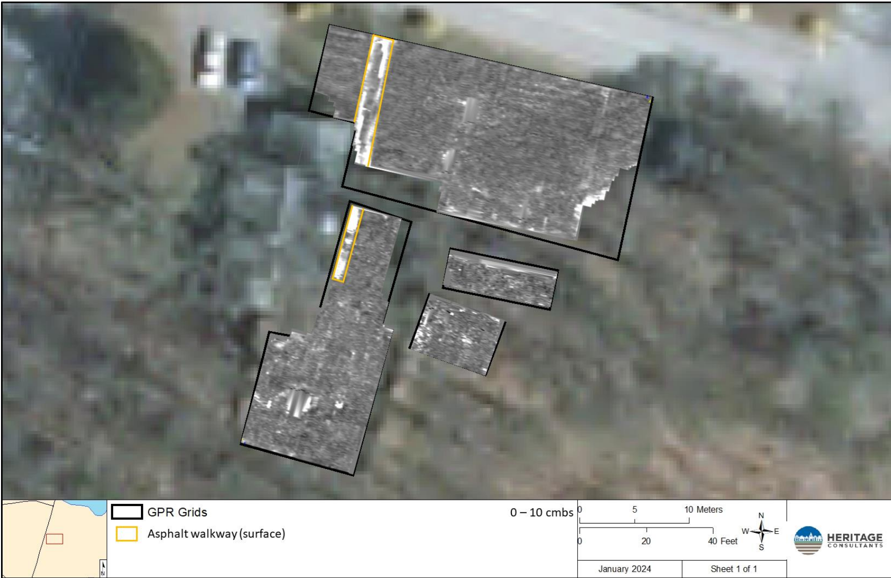
Figure 32: Annotated GPR amplitude map of Survey Grids 1-4, with approximate depth indicated.
