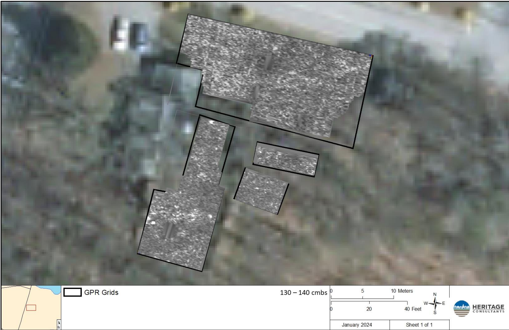
Figure 25: GPR amplitude map of Survey Grids 1-4, with approximate depth indicated.
