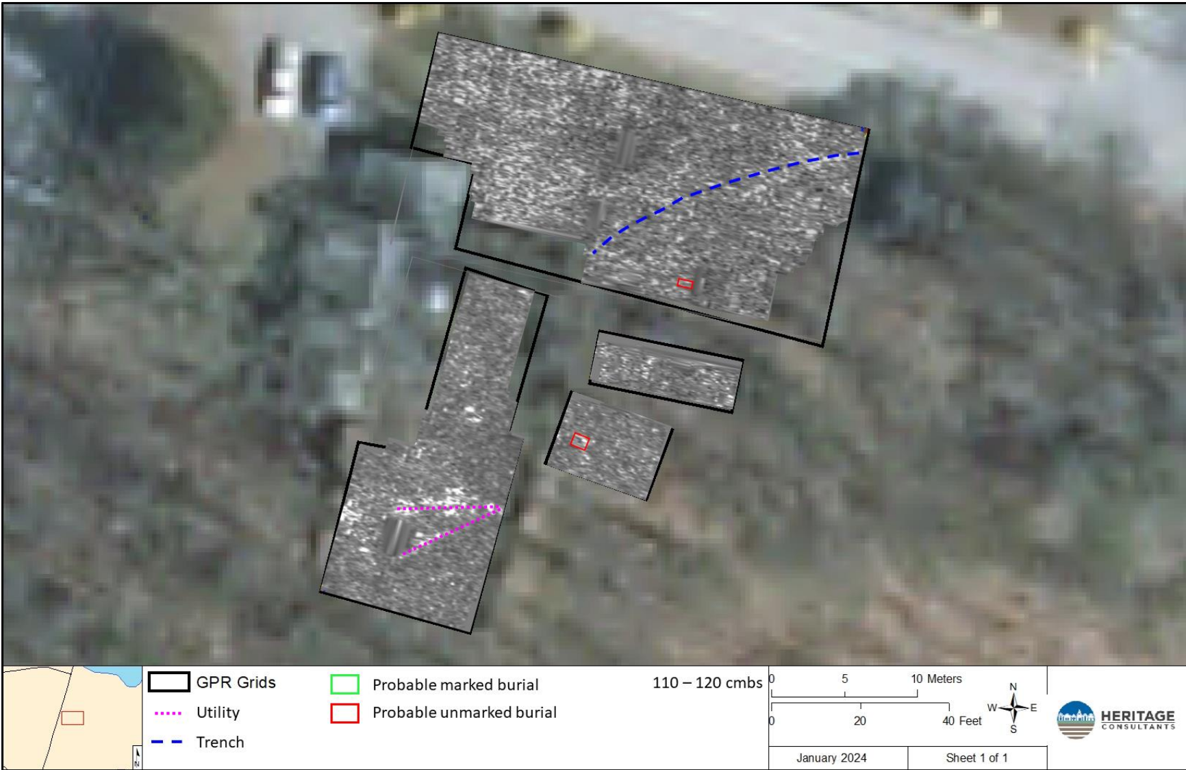
Figure 43: Annotated GPR amplitude map of Survey Grids 1-4, with approximate depth indicated.
