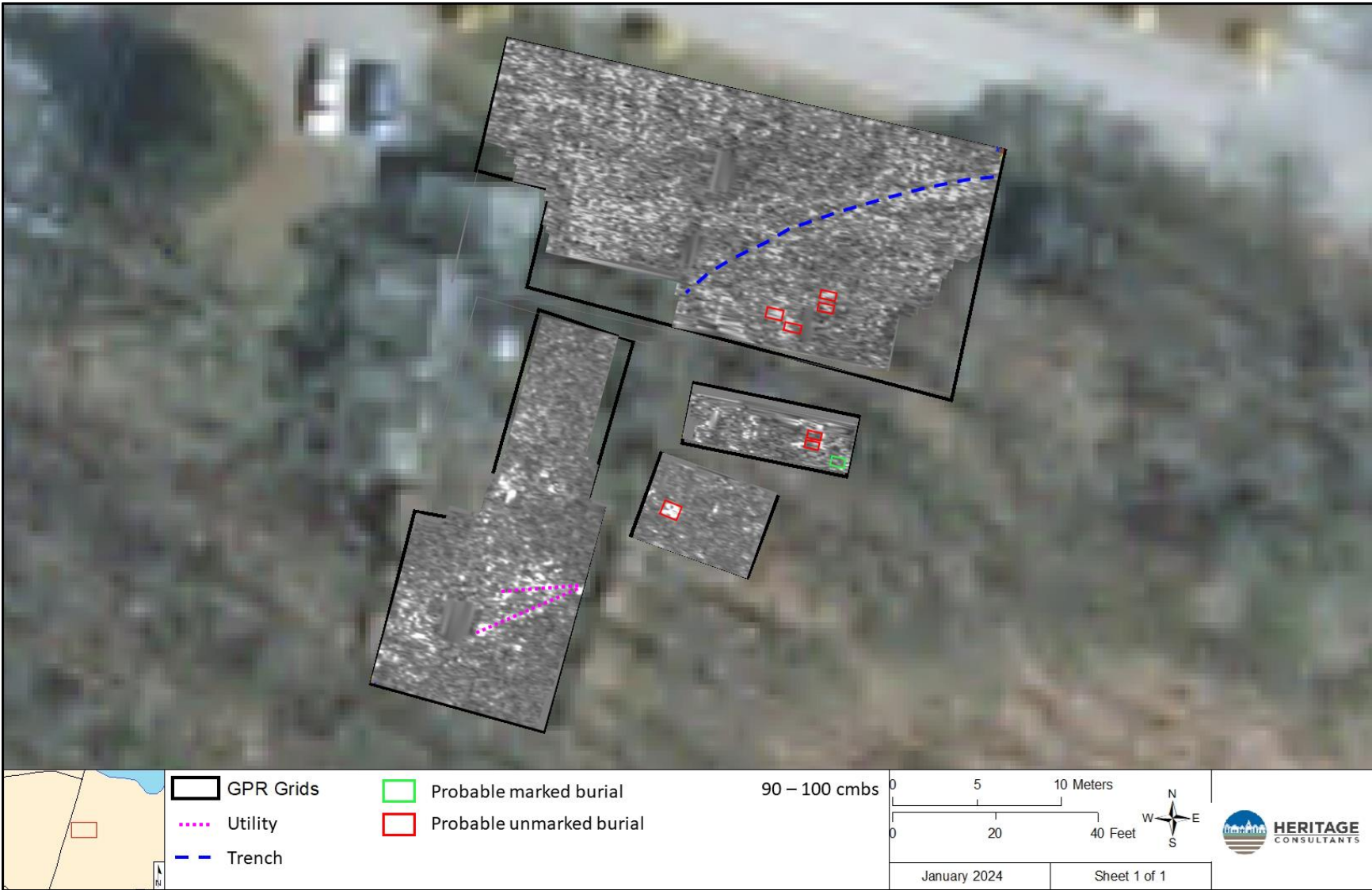
Figure 41: Annotated GPR amplitude map of Survey Grids 1-4, with approximate depth indicated.
