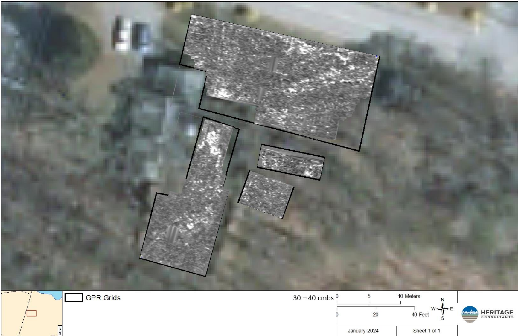
Figure 15: GPR amplitude map of Survey Grids 1-4, with approximate depth indicated.
