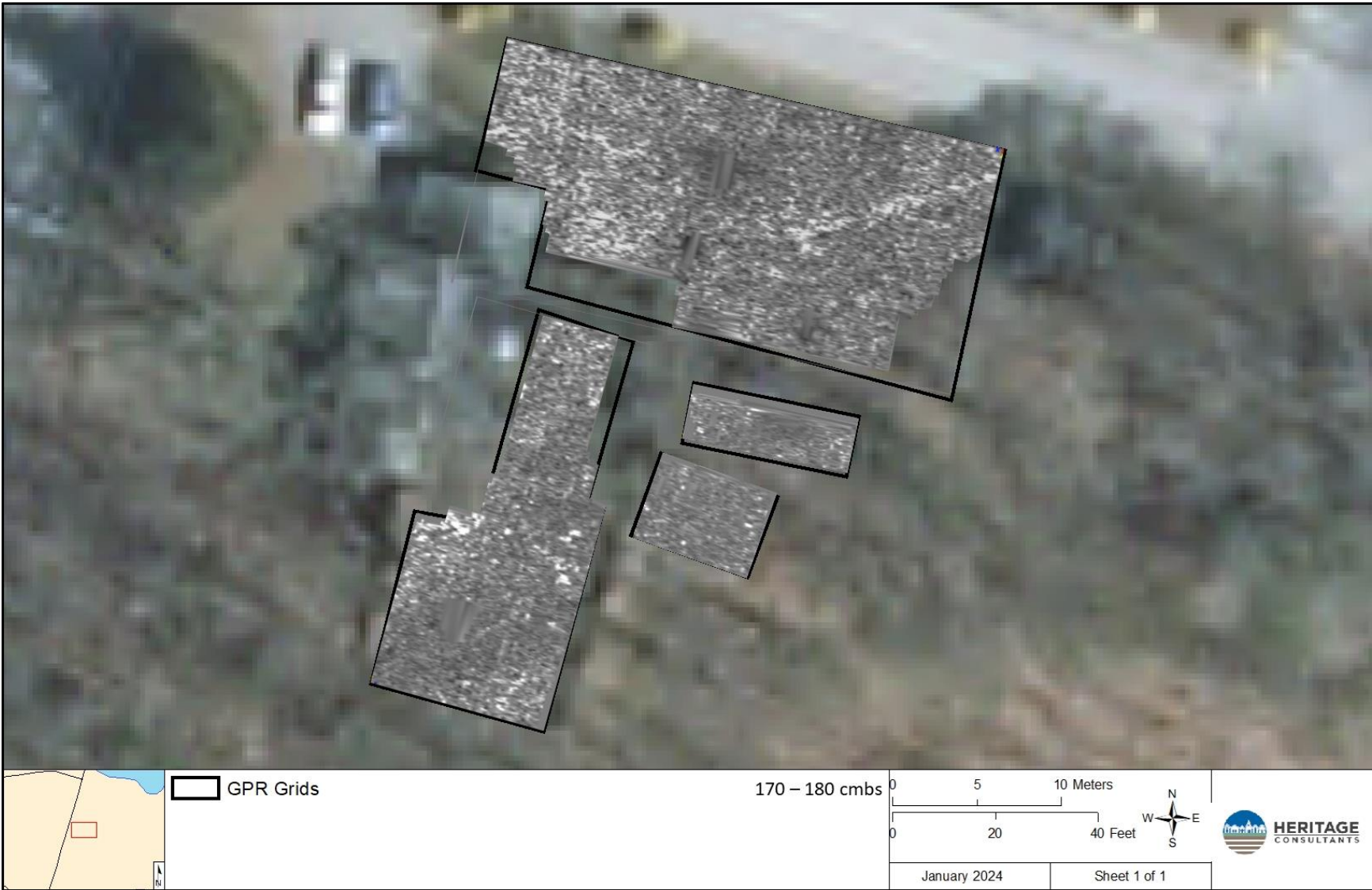
Figure 29: GPR amplitude map of Survey Grids 1-4, with approximate depth indicated.
