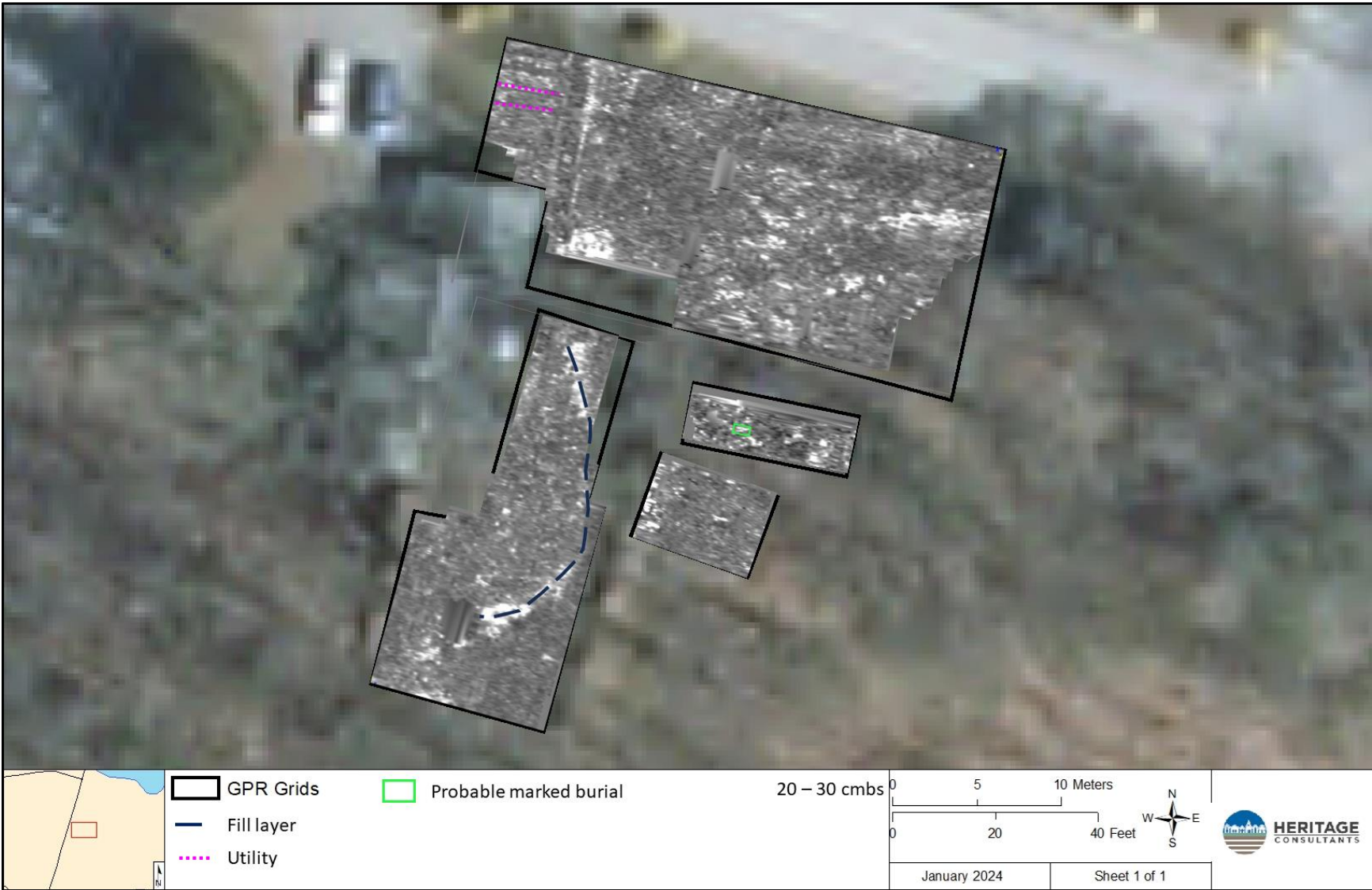
Figure 34: Annotated GPR amplitude map of Survey Grids 1-4, with approximate depth indicated.
