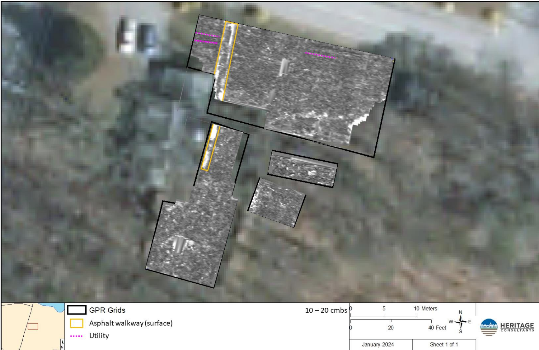
Figure 33: Annotated GPR amplitude map of Survey Grids 1-4, with approximate depth indicated.
