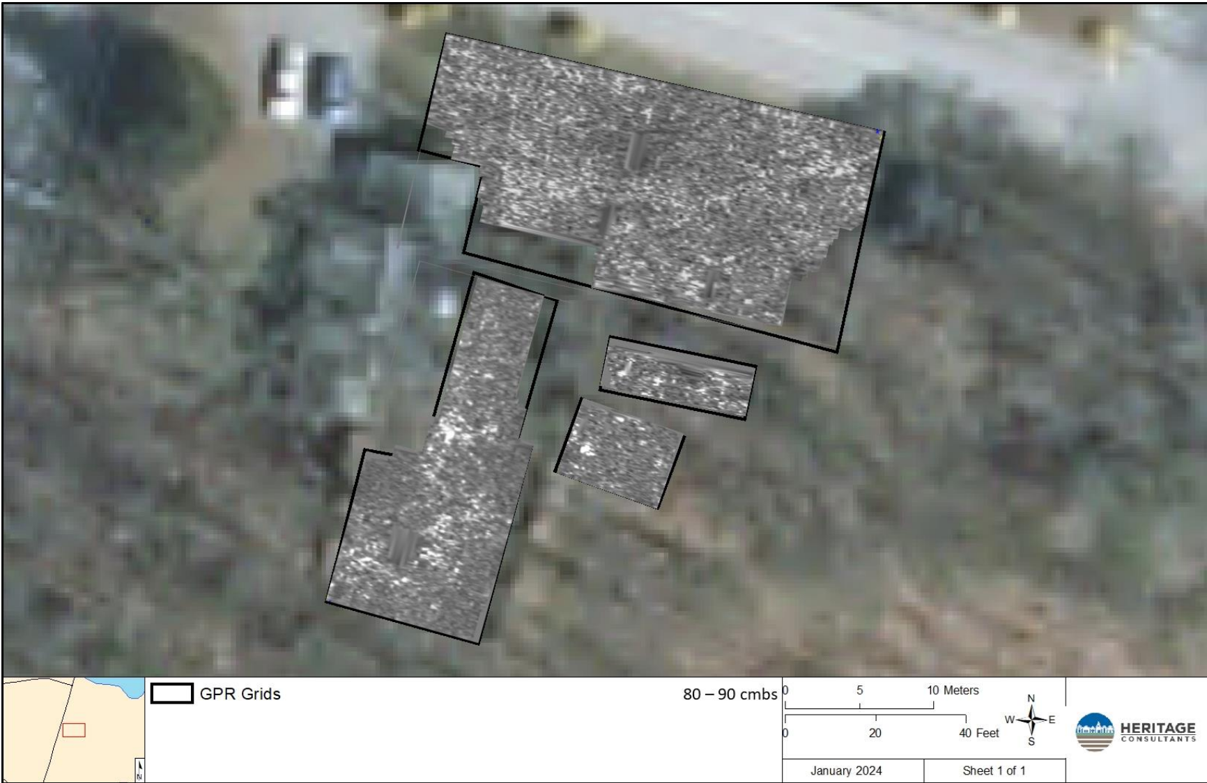
Figure 20: GPR amplitude map of Survey Grids 1-4, with approximate depth indicated.
