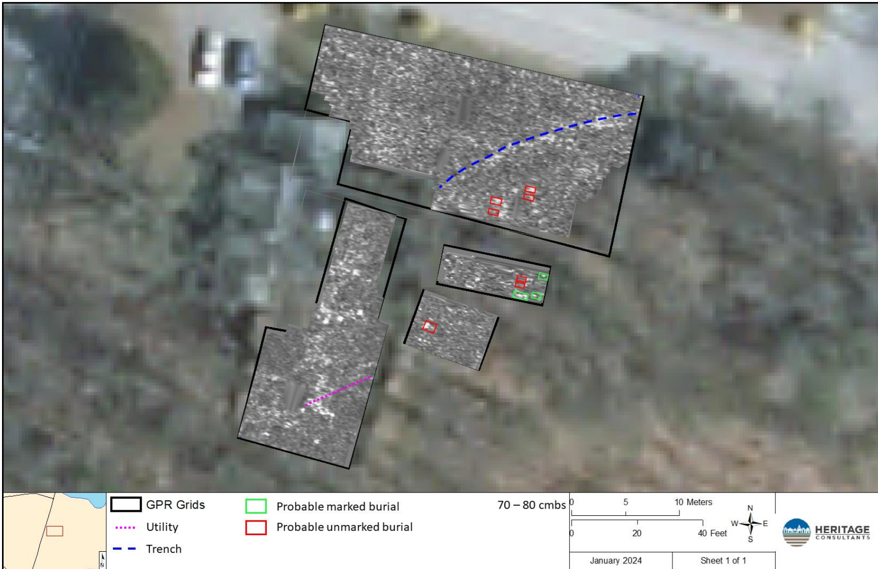
Figure 39: Annotated GPR amplitude map of Survey Grids 1-4, with approximate depth indicated.
