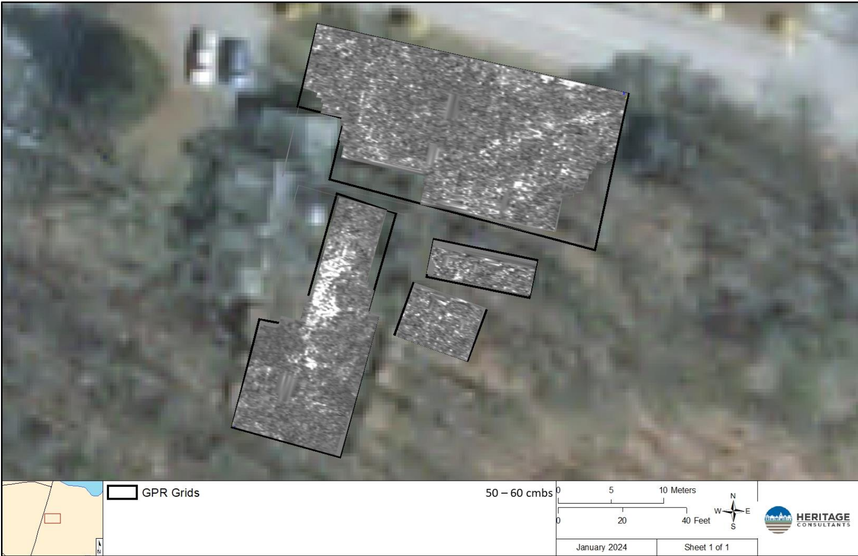
Figure 17: GPR amplitude map of Survey Grids 1-4, with approximate depth indicated.
