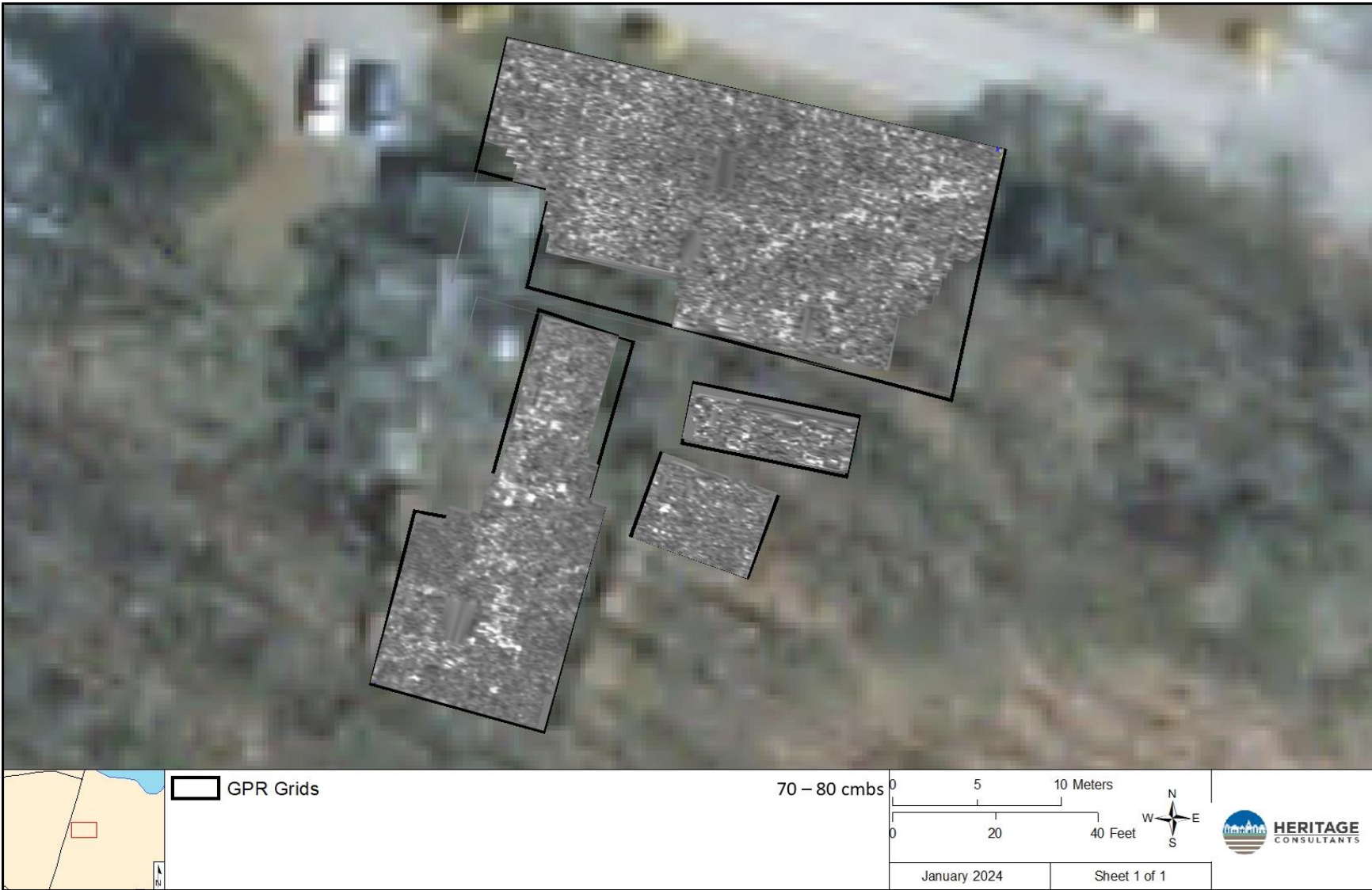
Figure 19: GPR amplitude map of Survey Grids 1-4, with approximate depth indicated.
