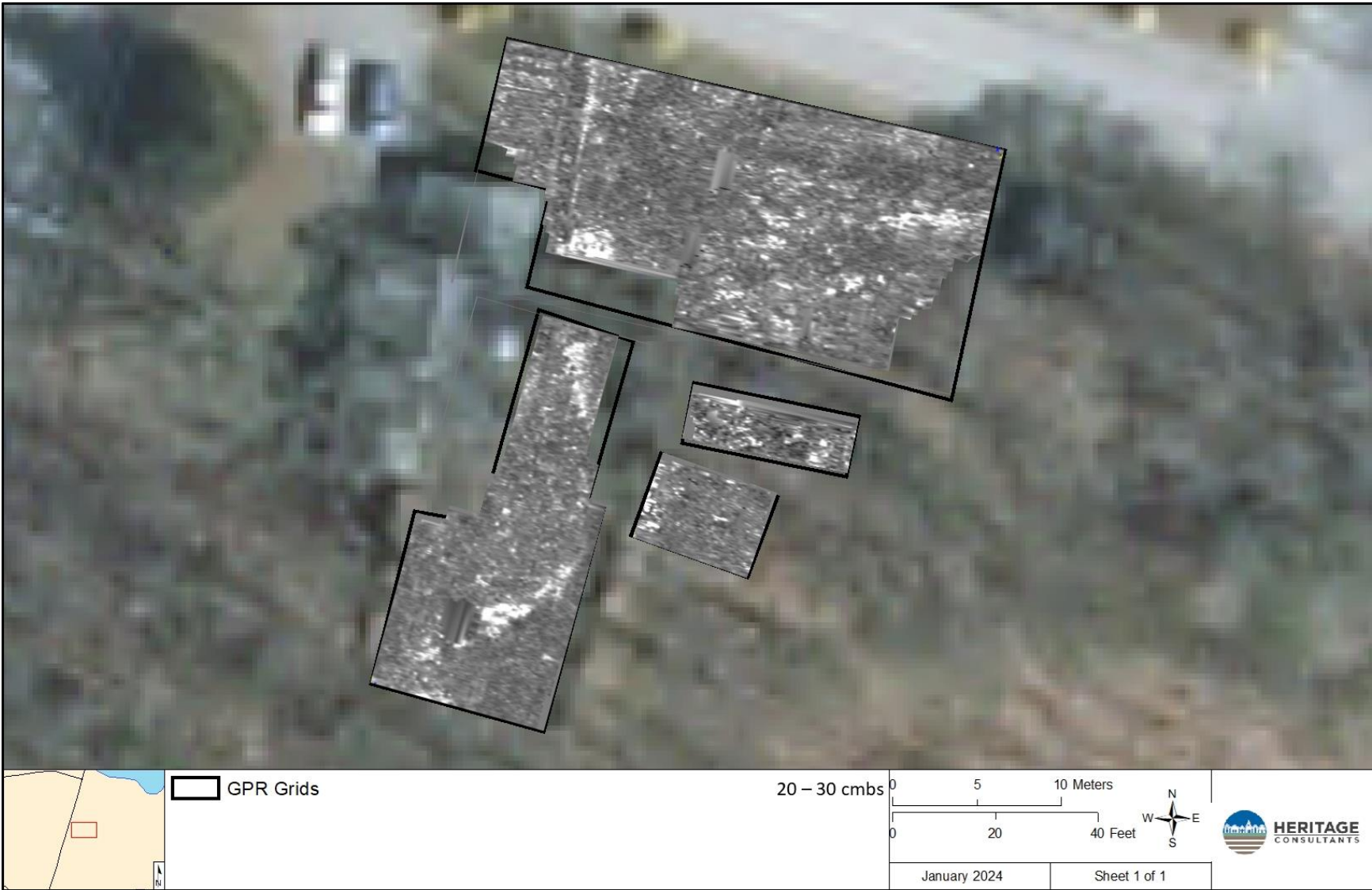
Figure 14: GPR amplitude map of Survey Grids 1-4, with approximate depth indicated.
