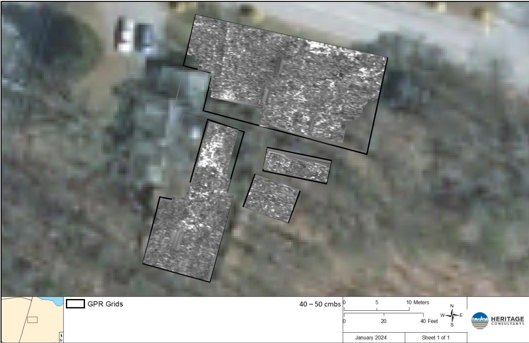
Figure 16: GPR amplitude map of Survey Grids 1-4, with approximate depth indicated.
