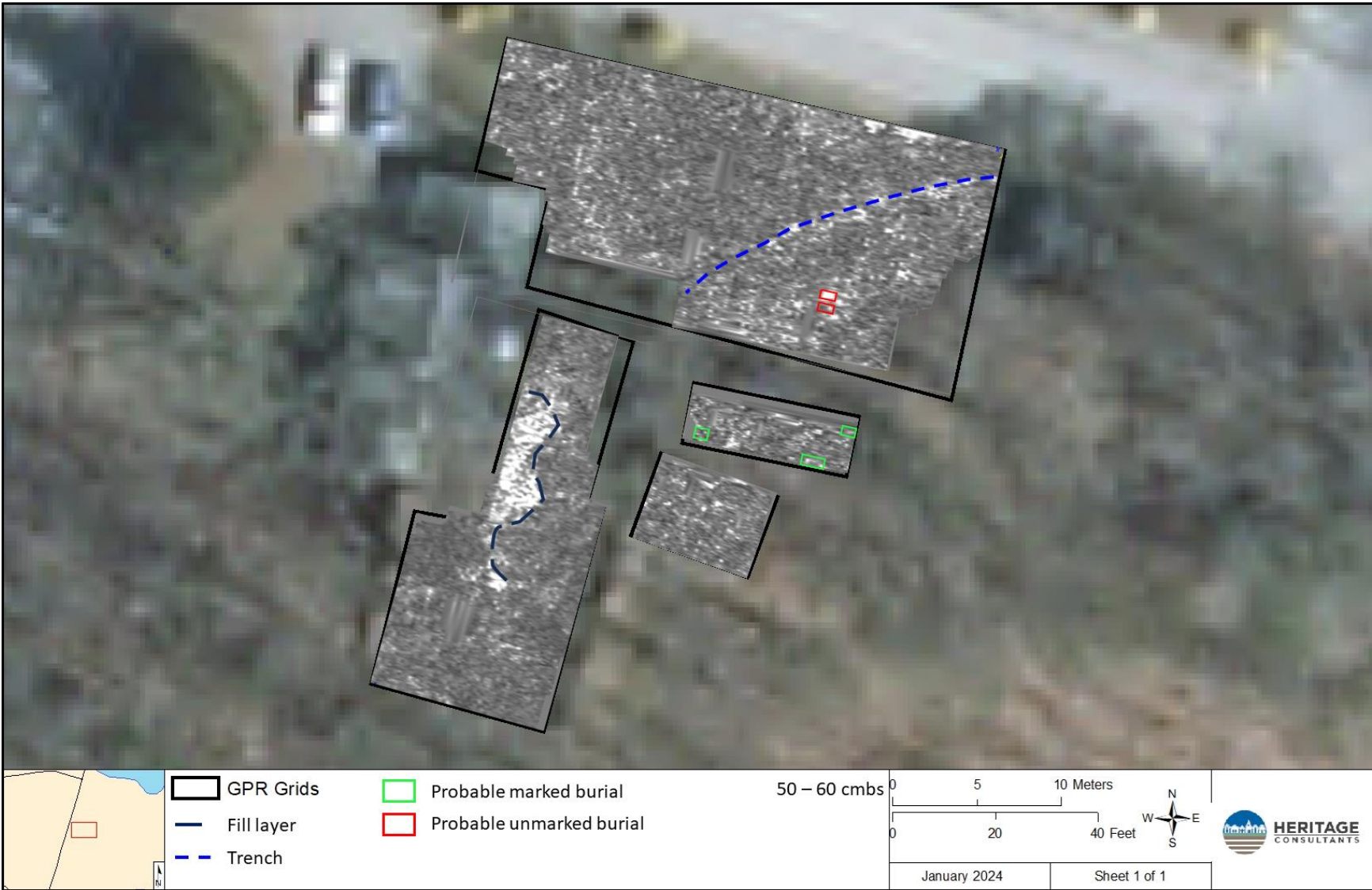
Figure 37: Annotated GPR amplitude map of Survey Grids 1-4, with approximate depth indicated.
