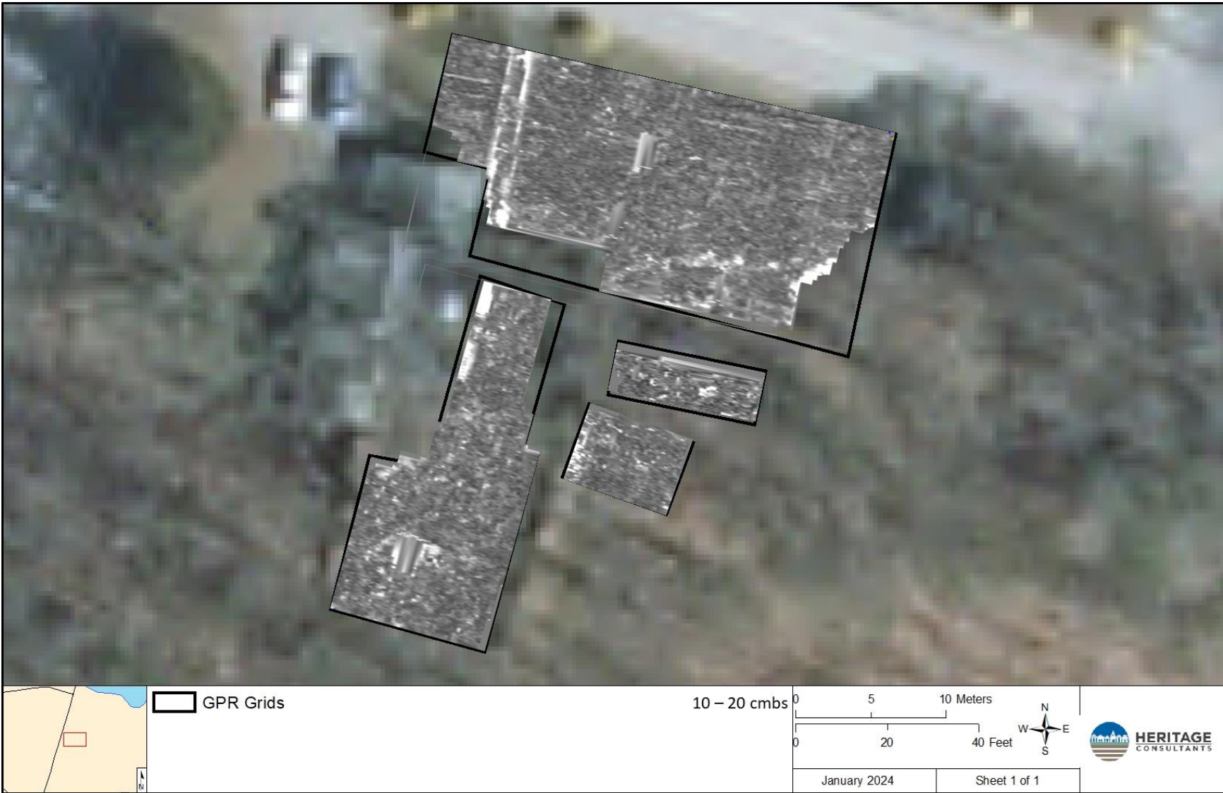
Figure 13: GPR amplitude map of Survey Grids 1-4, with approximate depth indicated.
