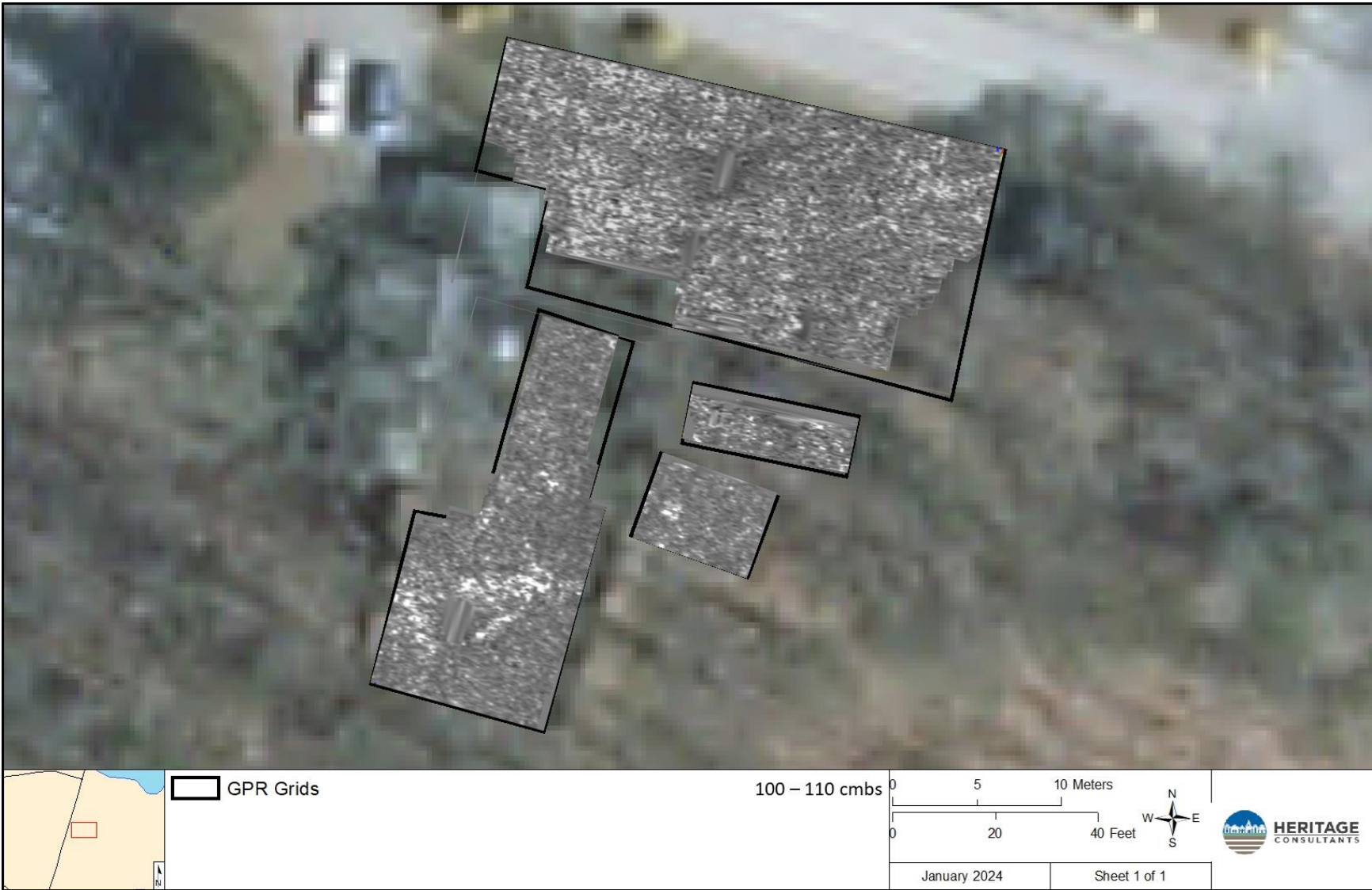
Figure 22: GPR amplitude map of Survey Grids 1-4, with approximate depth indicated.
