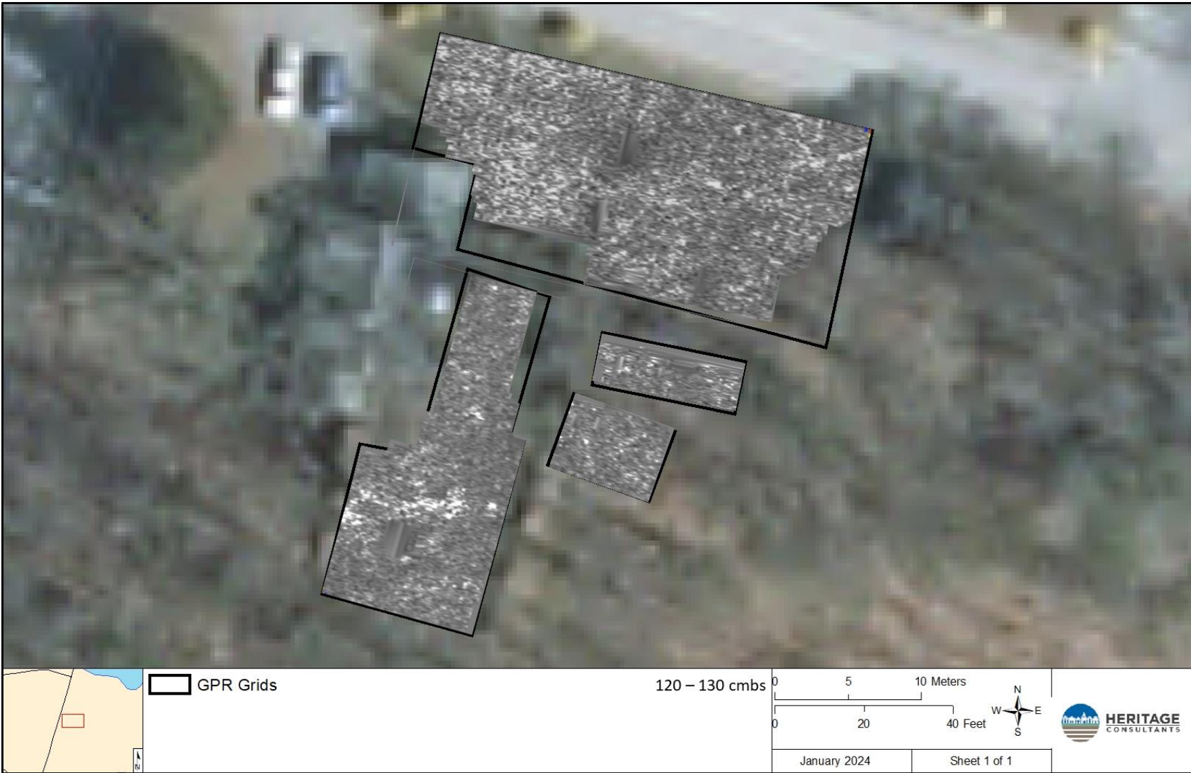
Figure 24: GPR amplitude map of Survey Grids 1-4, with approximate depth indicated.
