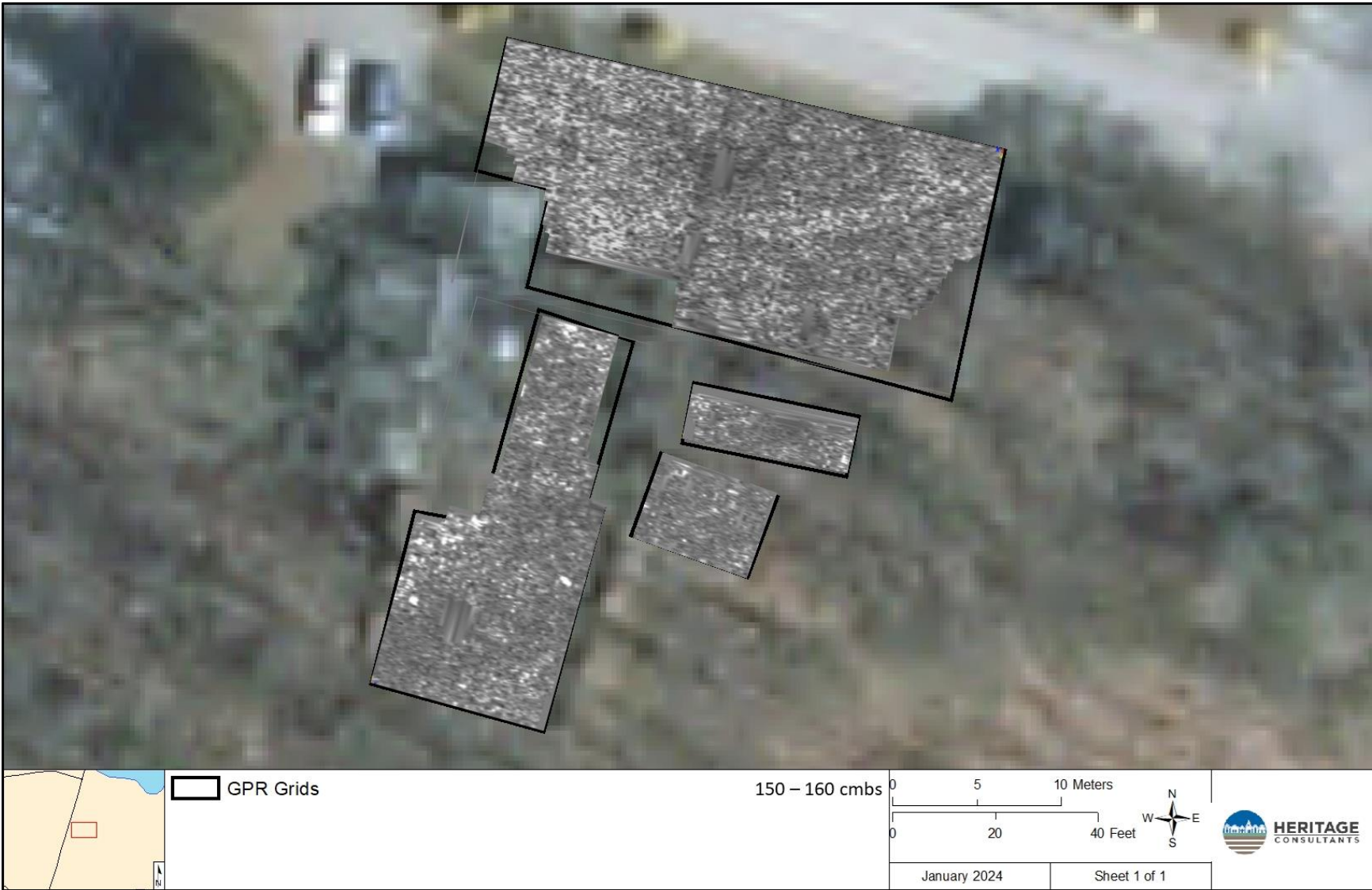
Figure 27: GPR amplitude map of Survey Grids 1-4, with approximate depth indicated.
