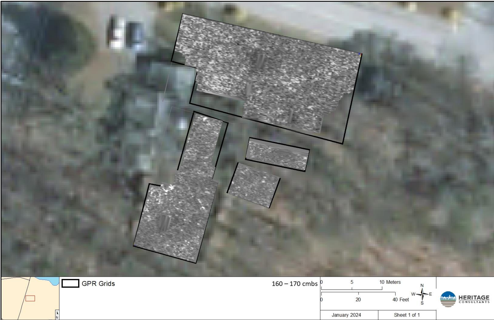
Figure 28: GPR amplitude map of Survey Grids 1-4, with approximate depth indicated.
