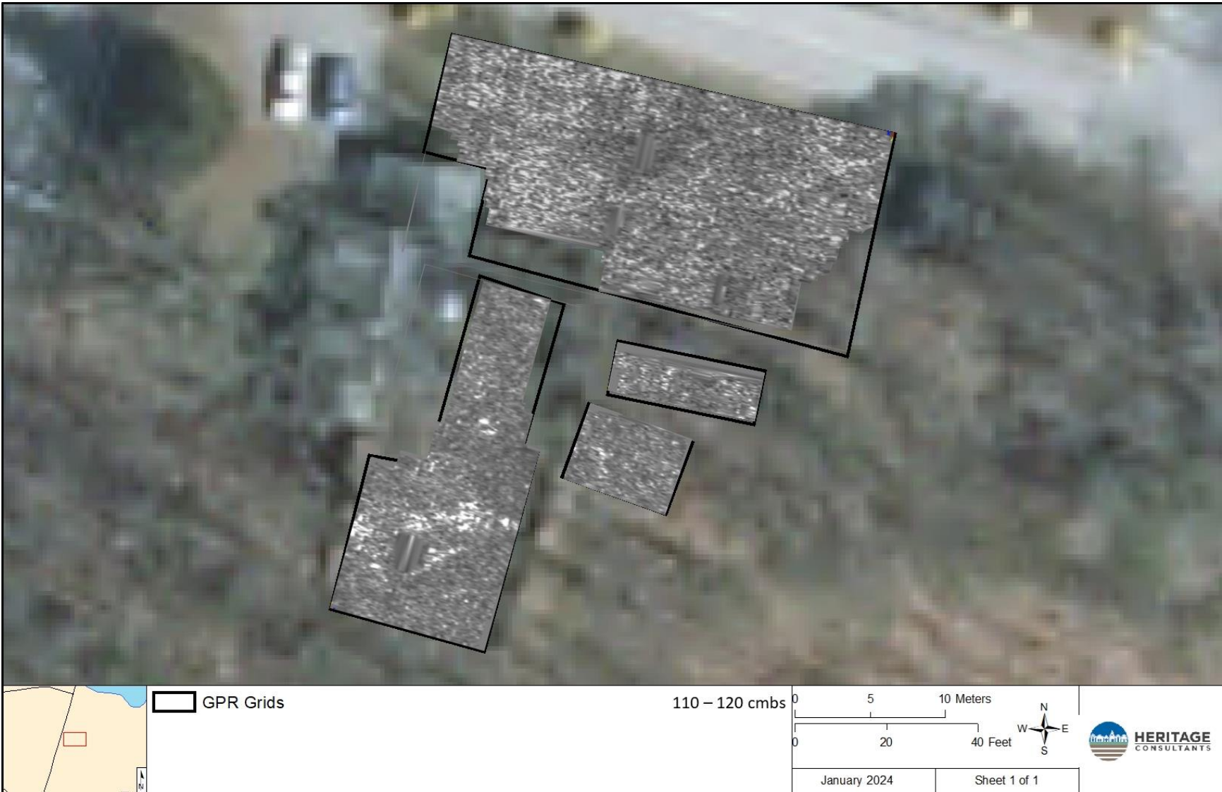
Figure 23: GPR amplitude map of Survey Grids 1-4, with approximate depth indicated.
