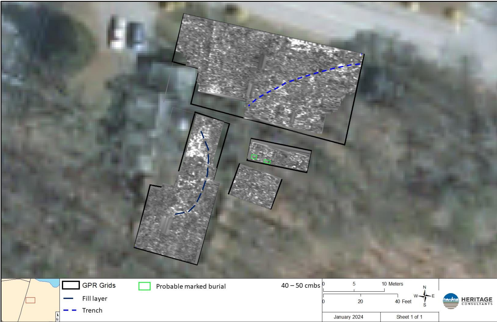
Figure 36: Annotated GPR amplitude map of Survey Grids 1-4, with approximate depth indicated.
