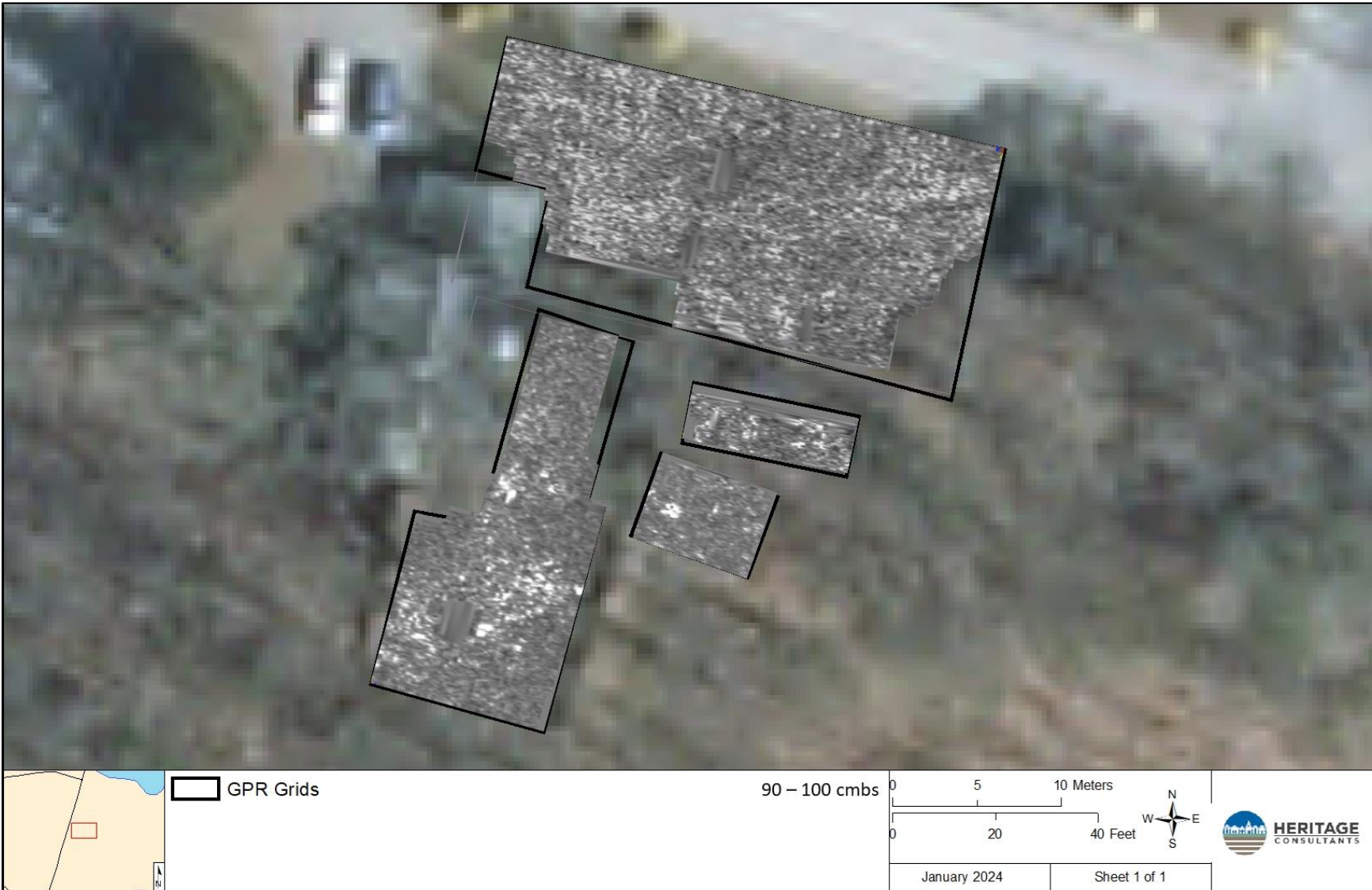
Figure 21: GPR amplitude map of Survey Grids 1-4, with approximate depth indicated.
