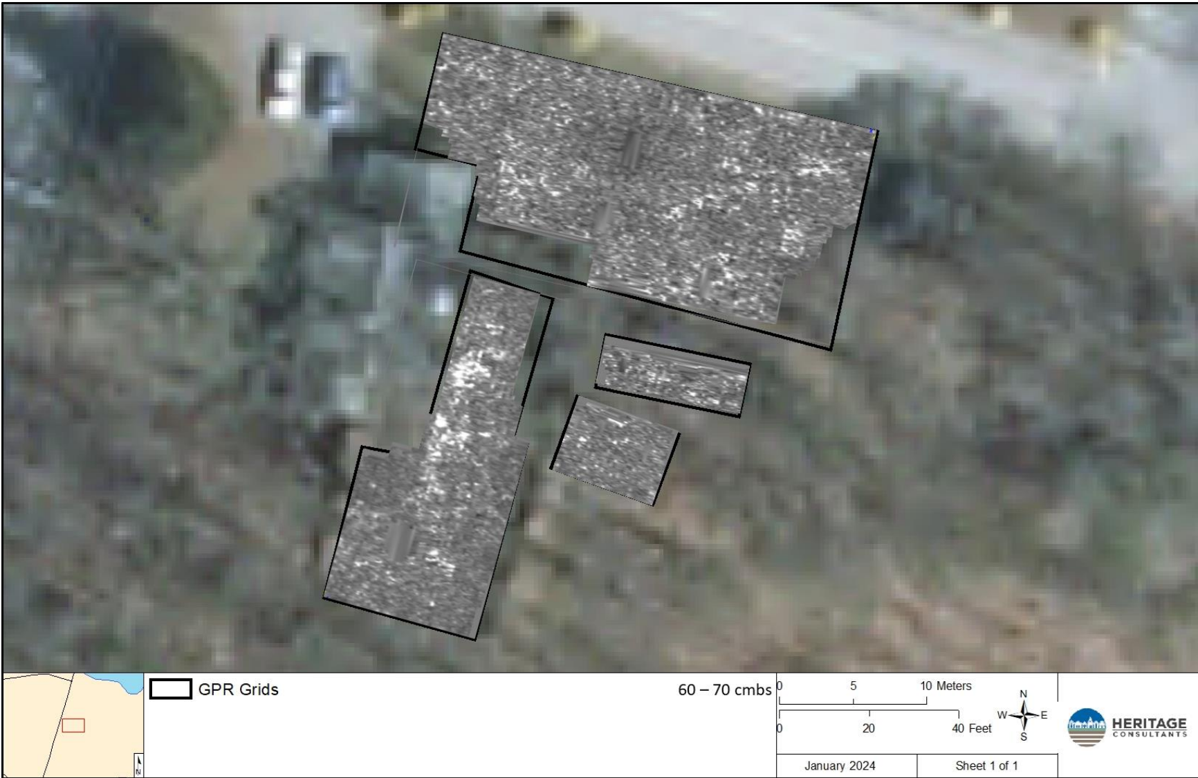
Figure 18: GPR amplitude map of Survey Grids 1-4, with approximate depth indicated.
